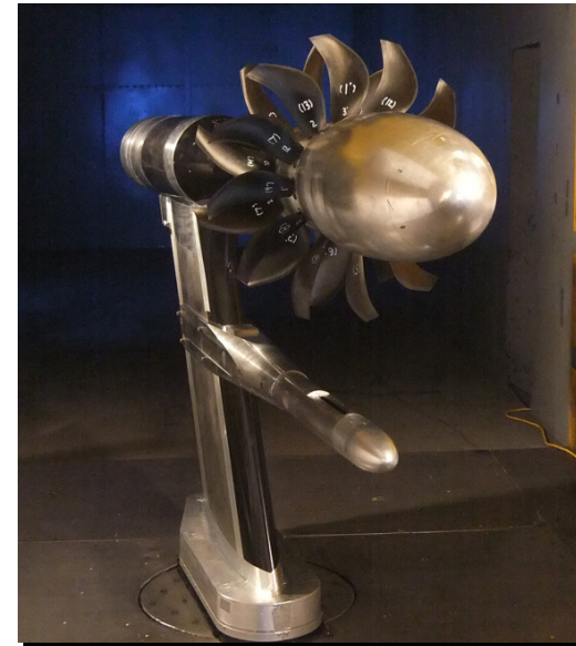
Model Scale GE HISTORICAL BASELINE Blade Set Installed in NASA Wind Tunnel
