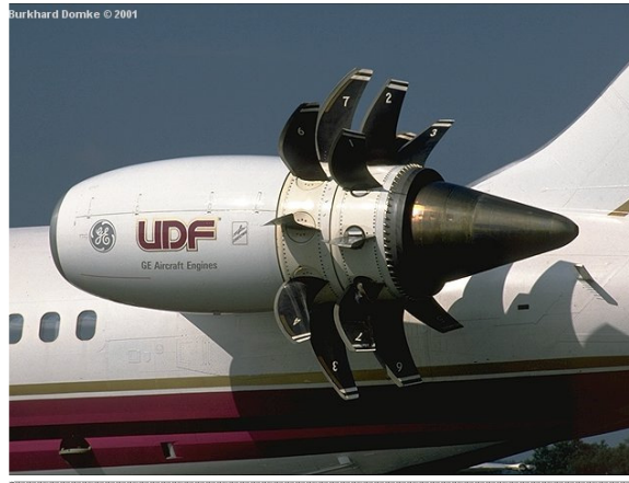
GE UDF Engine on MD-80 Aircraft (1987)
